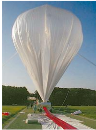
Figure 2: A Zero Pressure Balloon Used to Measure the Elements of the Atmosphere
