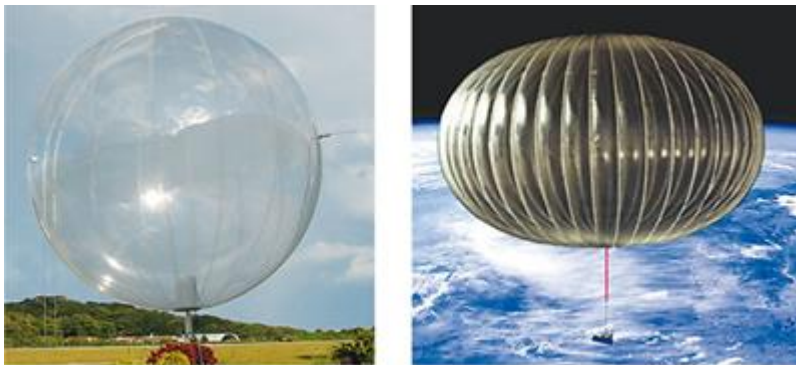
Figure 3: A High Pressure Balloon to Measure the Elements of the Atmosphere
