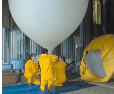
Figure 1: A Scientific Balloon Made of Synthetic Rubber
