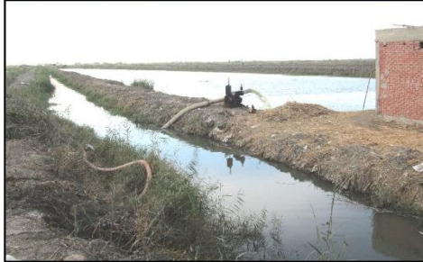
Fig. 11: Feeding Fish Farms with Water from Bahr El-Baqar Drain in the Study Area
